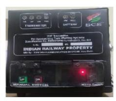
The above ATWS Transmitter should be installed at starting station of a section, and it should be connected with the Tx ON relay, operated through RRI cabin of the respective station.
